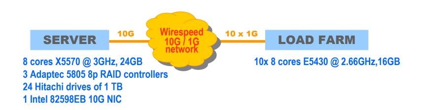
This setup reperesents well an elementary fraction of a typical large hardware installation and has basically no bottlenecks:
